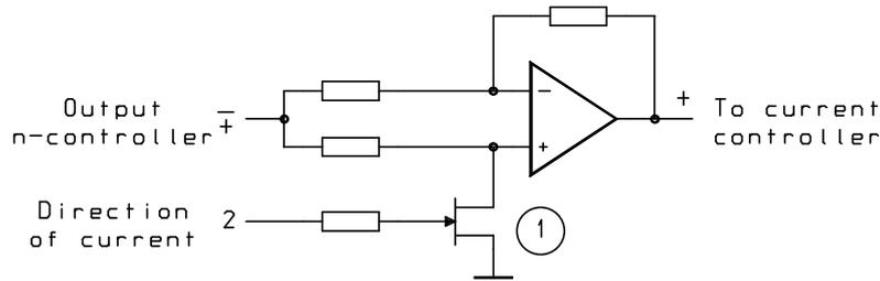
When thyristor bridge 1 is in operation, i.e. in motor mode with positive setpoint speed value (speed controller output negative), then the transistor (1) is conducting and the amplifier inverts the input voltage with the amplification  $-1$ . In the opposite current direction (speed controller output positive) the transistor (1) is inhibited and the amplifier does not function as an inverter with  $V = +1$ .
