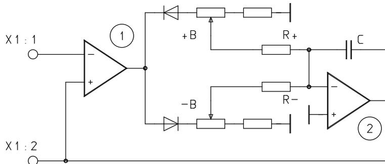
When a positive jump in setpoint value occurs at terminal X1: 1, the comparator (1) trips over to negative. Capacitor C becomes charged via resistance R+. The rate of charging is dependent upon the potentiometer setting +B. When the output voltage at the integrator (2) has reached the level of the setpoint value at X1: 1, the comparator (1) again trips over to 0 and capacitor C is no longer charged.
