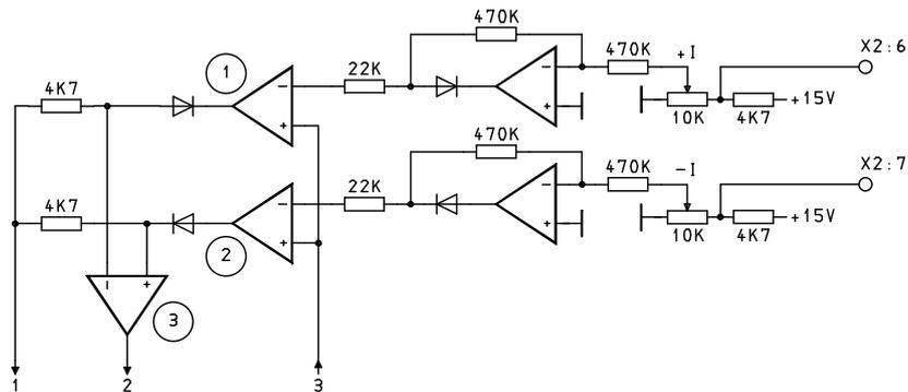
Comparators (1) and (2) are biased between 0 and 10V using potentiometers +I and -I. Comparator (1) is tripped over to positive, comparator (2) to negative. If the speed controller output (item 3) exceeds the set bias voltage, then the affected comparator trips over. The controller output is again taken back to the mixing point of the speed controller (item 1) via the corresponding diode and the relatively low resistance 4K7.
