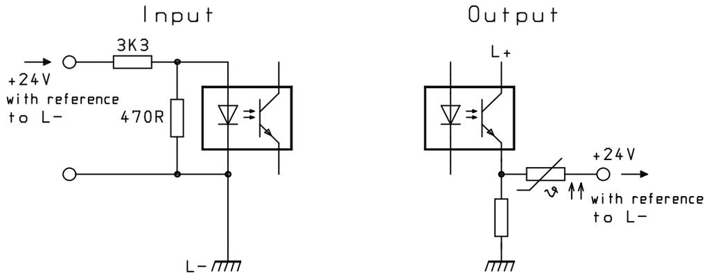
The reference potential -L, terminal X1: 14, is to be connected to the reference potential of the system control unit. It is recommended that the input and output wiring be shielded.
