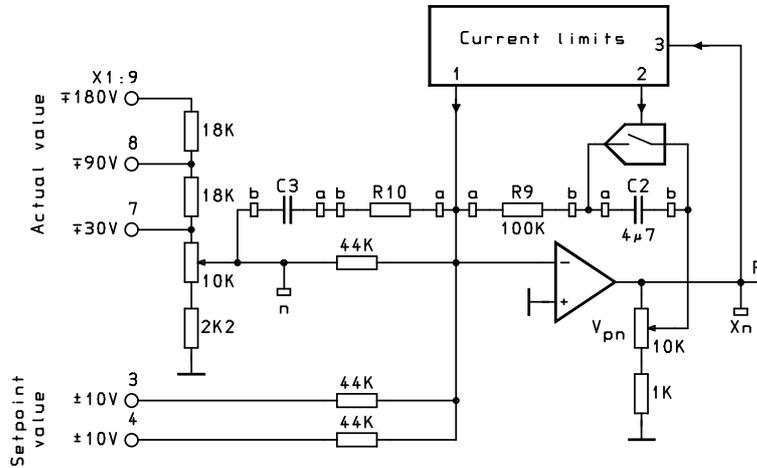
The speed controller is an ordinary closed-loop PI-controller. The proportional amplification is determined by R9 and potentiometer  $V_p$ , and the integral-action time by C2. The right stop of potentiometer  $V_p$  means the greatest amplification. The controller output can be measured at measurement test point "X." The PI-controller can be expanded to a PID-controller via C3 and R10. The actual speed, normalized to the setpoint value level, can be measured at measurement test point "n."
