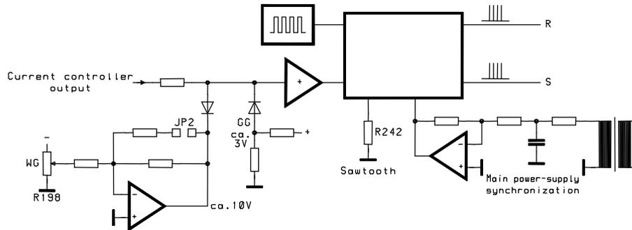
The integrated firing pulse element is controlled by the output voltage of the current controller. The firing pulses have a length of approx. 1 ms and are divided into 100 $\mu$ s-cycles. The rectifier limit (GG) is fixed, the inverter limit (WG) is set at the factory and may not be altered. For use with 60 Hz systems, the jumper JP2 must be placed on the open-loop controller circuit board.
