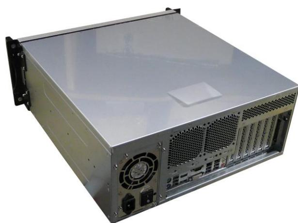
All of the components are designed for 24/7 continuous operation. The µATX-format mainboard is equipped with an additional USB port inside the case for the secure connection of e.g. a dongle. The power supply is a 300-watt industrial ATX PSU.
