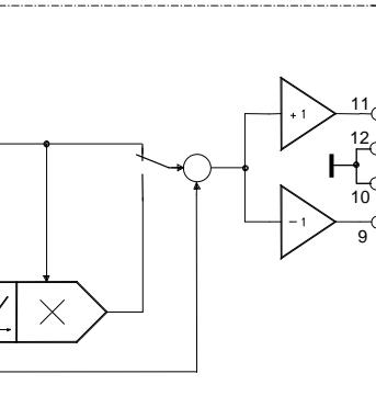
To form the difference between set value and actual value, the device has three equally valued inputs [1, 2, 3]. One of these inputs [1] operates invertingly. The connections can also be operated as current inputs (0/4 ... 20 mA) by closing the related switch. For actual value adjustment, one further input [4] with series resistor "R8" and adjusting trimmer "R5" is at disposal. For calculation "R8" use following formula (applies for "R5" in centric position):
